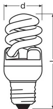
DTW 12 W/827 220...240 V E27, DTW 12 W/840 220...240 V E27, DTW 12 W/865 220...240 V E27
