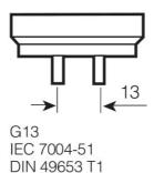
Tube diameter26 mmLength895.0 mmLength with base excl. base pins/connection895.00 mmDiameter26.0 mmMaximum diameter26.0 mm
