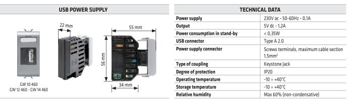
Not suitable for installation in boxes with a depth of less than 45 mm. If it is installed in a round box, the device should be positioned in the middle. To avoid any risk of overheating, the installation of several products side-by-side in one container is not allowed; insert a blanking module between two electronic devices.
