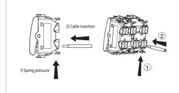
The spring terminals allow you to carry out the wiring in a shorter time, and without using screwdrivers or other tools. To insert the cable, it is necessary to press the orange lever (opening of terminal). Releasing the lever, the terminal closes automatically, firmly blocking the cable.
