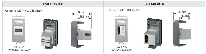
Given the depth of the adapters, when installed inside conventional flush-mounting and wall-mounting boxes, pay attention at the free space between the devices and the rear side of the box.
