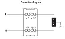
The Gewiss range to protect circuits against overvoltage in the domestic or similar environments includes the dischargers in the POWER catalogue, designed for installation in home enclosures.
