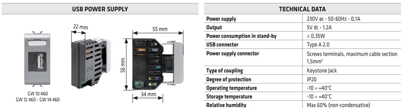
Not suitable for installation in boxes with a depth of less than 45 mm. If it is installed in a round box, the device should be positioned in the middle. To avoid any risk of overheating, the installation of several products side-by-side in one container is not allowed; insert a blanking module between two electronic devices.
