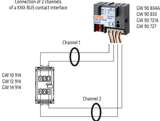
Connection to electronic control panel for moving roller shutters
