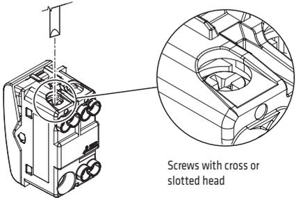
The terminals, located in the rear part of the devices, are manoeuvrable even after coupling the component to the support, and are suitable for both flexible and rigid cables. The components are supplied with the screws of the terminals open, to reduce wiring times.
