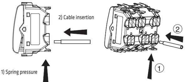
The spring terminals allow you to carry out the wiring in a shorter time, and without using screwdrivers or other tools. To insert the cable, it is necessary to press the orange lever (opening of terminal). Releasing the lever, the terminal closes automatically, firmly blocking the cable.
