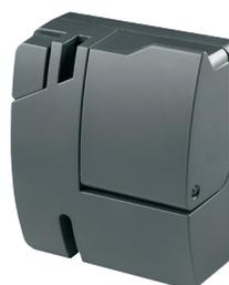
The wireless water sensor should be positioned in line with the floor in order to reveal the presence of any type of liquid. To allow it to work correctly, when positioning the probe you must bear in mind the slope and/or probable leak localisation points (e.g. under sink, etc.) The sensor must be positioned so that the LED is visible and the push-button accessible.
