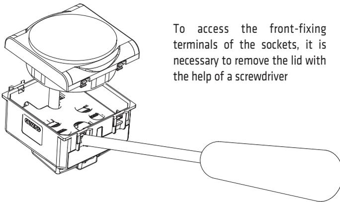
To access the front-fixing terminals of the sockets, it is necessary to remove the lid with the help of a screwdriver
