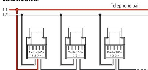
• The clamps 3 and 4 are connected by means of the contact inside the telephone, which is closed when the telephone receiver is put down. When the telephone receiver is picked up, the line breaks downstream (L1 pole), ensuring that the conversation is not overheard.
