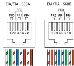
To obtain the EIA/TIA 568A or 568B configuration shown alongside, follow the colour code given on the terminal block (of the products).
