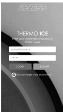
Press the **LOGIN** button key. The page for configuring the network parameters will appear. Enter all the data relating to the domestic wireless network to which THERMO ICE will connect in order to communicate with the remote server (via the Internet).
