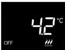
The **anti-freeze function** is only active in heating mode, when the temperature adjustment system is switched OFF. In this case, the thermostat uses anti-freeze temperature setpoint, reactivating the heating system only if the room temperature falls below  $T_{ANTI-FREEZE}$ .
