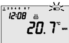
When the batteries charge is low, the symbol on the display starts to blink. Operation of the timer-thermostat is guaranteed in any case. In this case, the batteries must be replaced as soon as possible.
