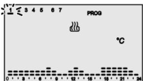
The PROG symbol appears on the display while the bar for the first day of the week will start to blink. Select the first day required with keys **(-) (+)**. Press key **(○)** within 30 seconds to confirm the selection.
