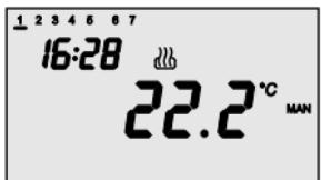
In **manual operation** the timer-thermostat permanently uses a temperature set point that can be freely set. The text MAN and the ambient temperature measured appear on the display.
