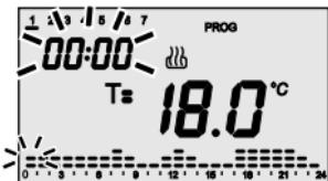
After confirmation of the first day, the current profile, relative to the day selected is displayed on the display. The hour starts to blink. Select the temperature set point that it is required to set starting from hour 00:00 using keys **^ V**.
