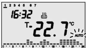
Activation of the forcing is signaled on the display by the blinking of the AUTO symbol.
