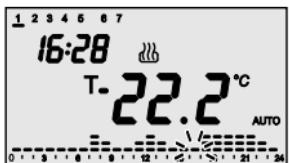
In **automatic operation** the timer-thermostat uses a program that can be different for every day of the week. The text AUTO, the ambient temperature measured and the symbol of the set point relative to the current quarter of an hour appear on the display.
