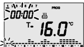
The symbols **T<sub>-</sub>**, **T<sub>s</sub>** or **T<sub>e</sub>** and the value corresponding to the selected set point appear on the display. The set point is applied to the hourly profile until the first variation present in the current program.
