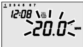
To activate manual operating mode, press key  $\odot$ , until the text MAN appears on the display. The temperature set point appears for about two seconds. Use keys  $\wedge \vee$  to set the required set point value, press key  $\odot$ , or wait 5 seconds to confirm the setting.
