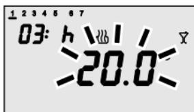
Press key  $\textcircled{Y}$ , to activate the function, the symbol  $\textcircled{x}$  appears on the display while the value of the set point active at that time starts blinking. Use keys  $\wedge \vee$  to set the new value of the temperature set point.
