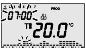
Increase the time with keys **(-) (+)** until the moment when it is required to modify the proposed profile; during the increase the column relative to the selected time blinks on the hourly profile. Select the new set point with keys **^ V**, which will be applied until the next variation present in the program.
