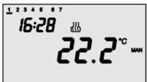
Dans le **fonctionnement manuel** the timer-thermostat permanently uses a temperature set point that can be freely set.
