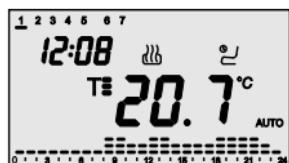
When the day selected for the feast copy is in progress, symbol is fixed on. The validity of the feast day copy is temporary, after midnight of the selected day, a return is made to the programmed weekly profile.
