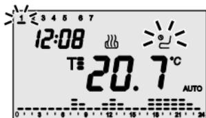
When the function is active, pressing key displays the day to which the feast day profile has been copied: the corresponding bar starts blinking on the display. Press key ; again to deactivate the function; if it is required to modify the day of the week, use keys and press key , or wait 30 seconds to confirm the new setting.
