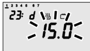
Press key to activate the function, the symbol appears on the display while the value of the set point active at that time starts blinking. Use keys to set the new value of the temperature set point.
