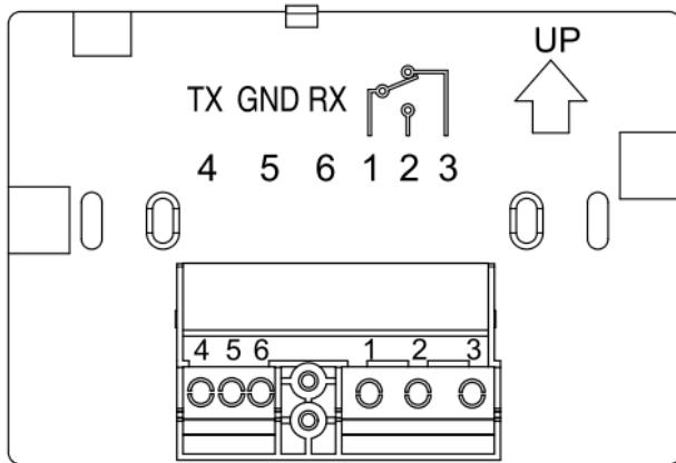
Remote control unit connection (serial line).
