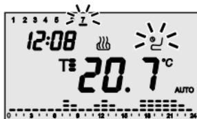
Press key , to activate the function, the symbol and the bar of the feast day start blinking on the display. Use keys to select the day of the week to which to copy the feast day profile; press key , or wait 30 seconds to confirm the setting made.
